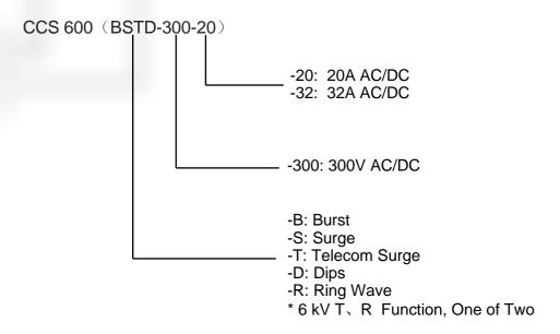
Note: Pulse magnetic field, power frequency magnetic field, drop accessories, coils, external networks and other accessories have independent models and are not reflected in the host model.
