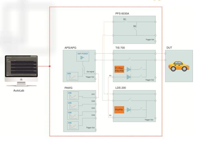
The PAWG signal generator shown in the above figure has been embedded in the APS xxxxDSR series instruments, improving integration and facilitating the layout of the test site.
